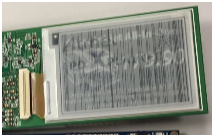
Figure 3 - Screen with vertical lines
