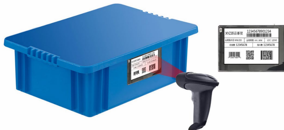
Figure 10 - E-paper displays can be scanned with a reader and are ideal for logistics applications
