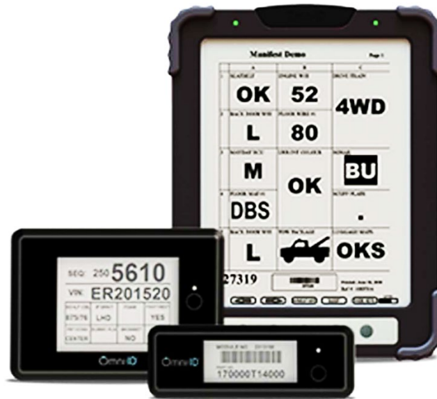
Figure 7 - E-paper complements RFID by making the data stored on the tag human-readable.
