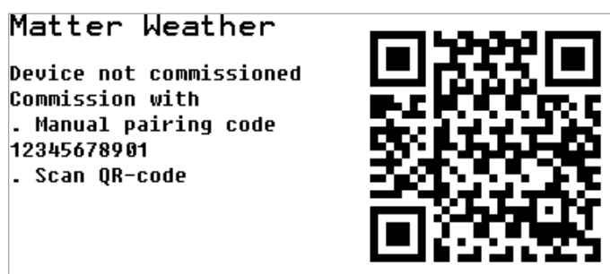
Figure 10 - The e-paper display plays a critical role for a fast and secure Matter commissioning
