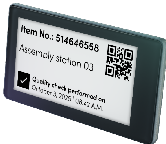
Figure 7 – This batteryless smart tag combines NFC technology with an e-paper display (Source: PDi-Digital GmbH)
