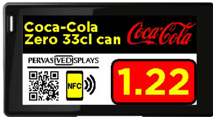
Figure 5 – This Electronic Shelf Label powered by a Pervasive Display EPD has excellent readability and a 10-year above battery life (Source: Vusion Group)
