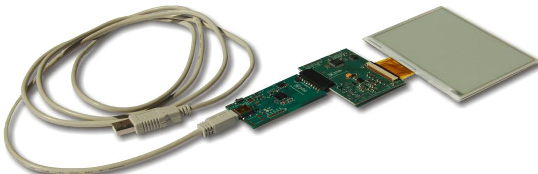
Figure 2.2: USB2TCM\_v1.1 connected to a TCM-P441
