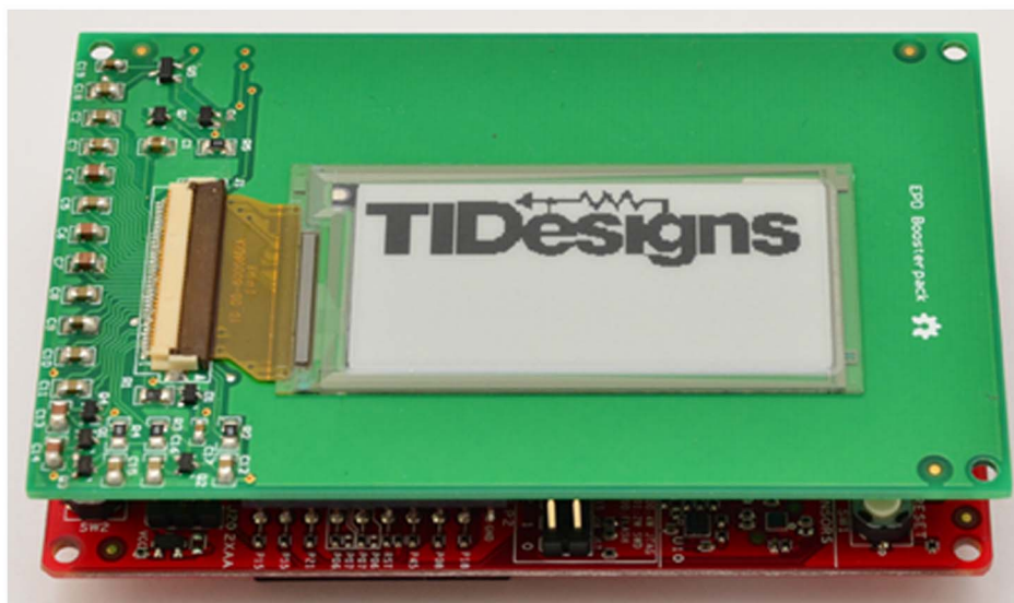
Fig 8. TI's CC3200-based EPD reference design can be updated over local wireless networks or through the cloud, using MTTQ.
