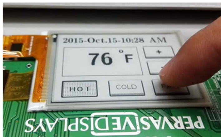
Fig 4. This 2.7-inch eTC e-paper module with capacitive touch overlay, demonstrates a responsive user interface for a thermostat, implemented using partial updates.
