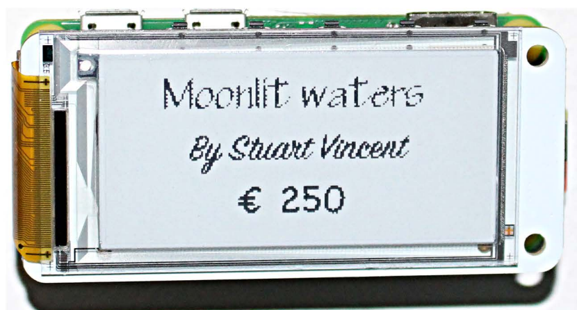
Figure 6 – PaPiRus Zero and Raspberry Pi Zero W used for art gallery application
