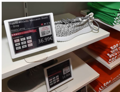
Figure 2: Electronic shelf labels are easy to update, can use color to highlight text and also display QR codes.
