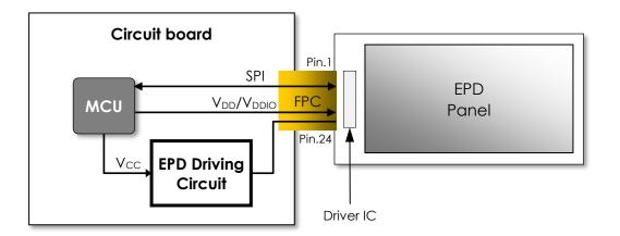
Please follow the EPD driving circuit below on your PCBA to work with our EPD panels for iTC drivers. All the components and circuits are necessary.
