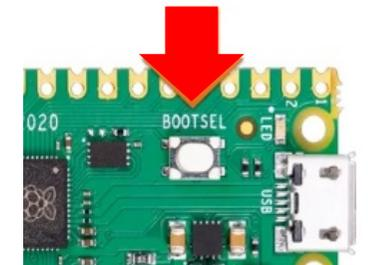
8. Release **BOOTSEL** button once the new storage device named **RPI-RPI2** appears in the computer.
