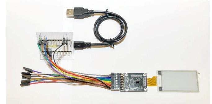
7. Press down the **BOOTSEL** button (right) on the Pico and hold it while you connect the other end of the micro USB cable between the Pico and your PC. This installs your Raspberry Pi Pico as a mass storage device named **RPI-RPI2**.
