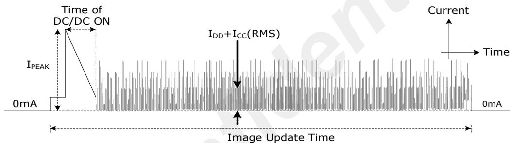
The "Time of DC/DC ON" which contains the some current peak of  $V_{GH}/V_{DH}/V_{GL}/V_{DL}/V_{COM}$ .
