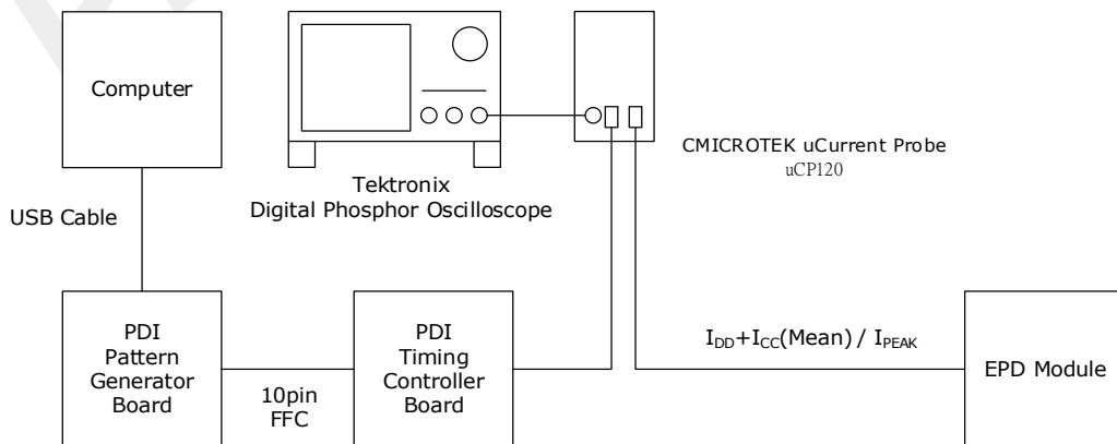
\*Set oscilloscope filter > 200MHz and record length to 10M points.
