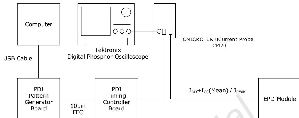
\*Set oscilloscope filter > 200MHz and record length to 10M points.
